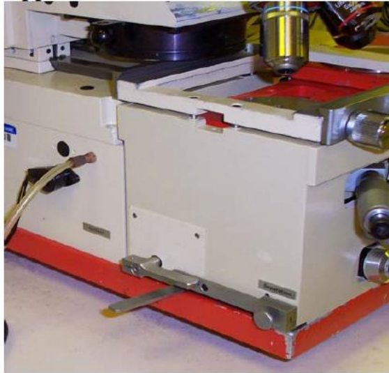
Figure 7 Contact Lever (rotation shown in chuck lowered position ) and Separation Lever (Slide shown in contact position)
