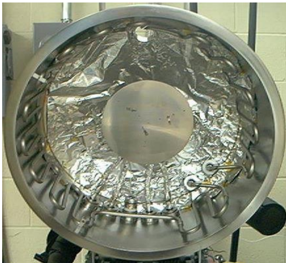
Figure 2: Lid Interior Lid Sample holder in the center and cooling coils on the outer edge of the lid.
