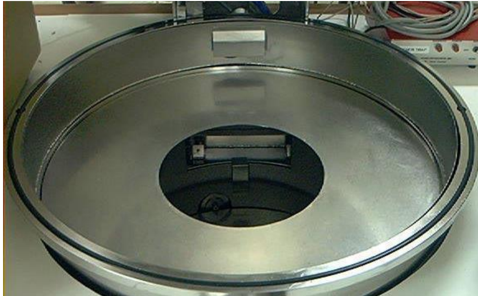
Figure 3: Gate restriction plate; To protect the lid interior never start beam without this in place.
