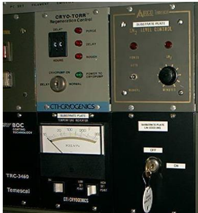
Figure 5: Regeneration Control (Top Left) And LN controls (Bottom and top Right).
