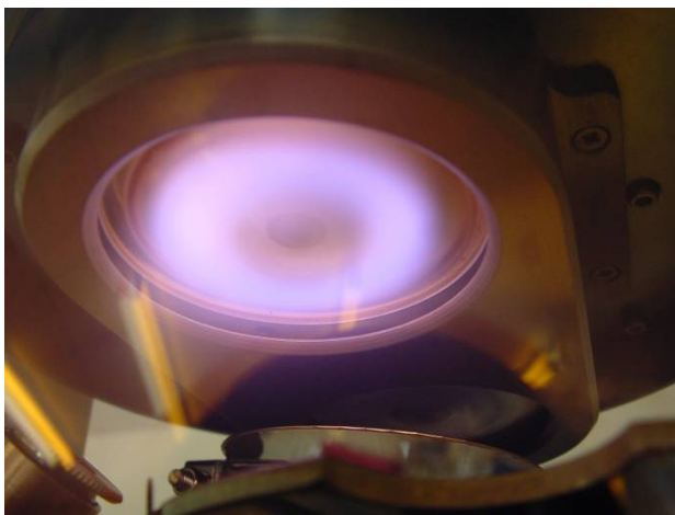
Figure 5-4: Desired Plasma Formation
