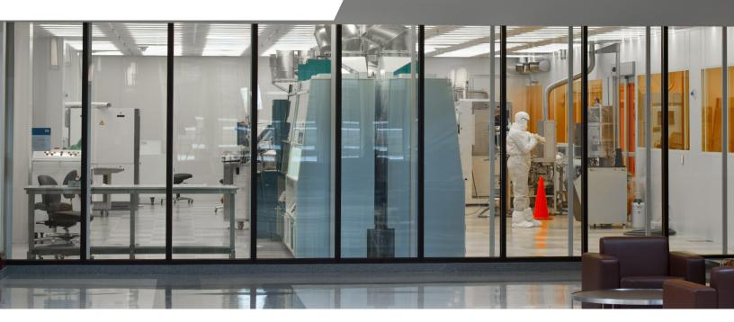
The Notre Dame Nanofabrication Facility is the equipment set and supporting cleanroom environment for research and teaching in nanoelectronics, optoelectronics, microfluidics, nanofabrication, and related disciplines. The facility consists of a 9,000 square foot clean room and a full complement of processing and test equipment necessary for fabricating and analyzing the performance of advanced devices.
